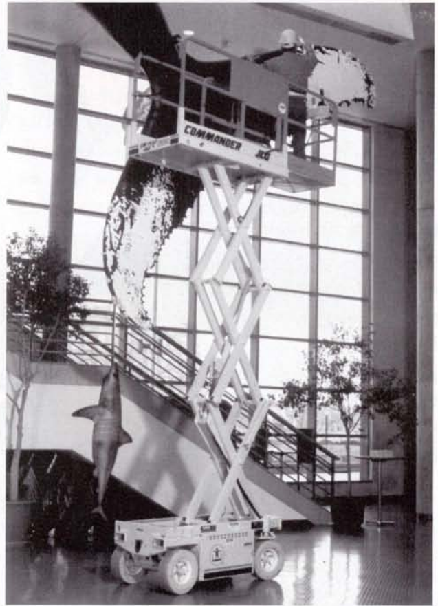
JLG's new 4.3 metre (14 foot) Mini Scissor Lift is designed for the tightest work environments with an overall width of only 0.81 metres and low retracted height of 1.52 metres.
